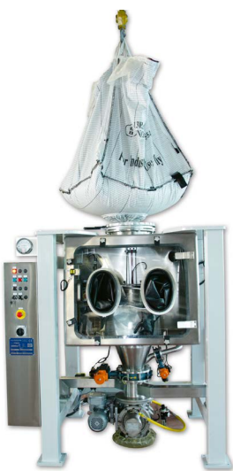
Big-Bag emptying with endless-foil system in a glove box
