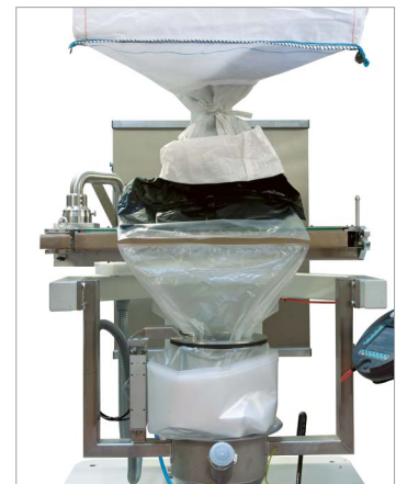
SMART Containment – peelable containment-foil, exclusively available from Novindustria
