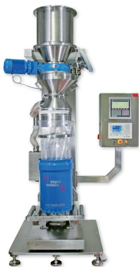
Single bag filling with Novi-Dos®
