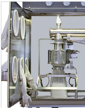
Dosing and filling system with endless-foil and thermal cutting/welding equipment in the isolator
