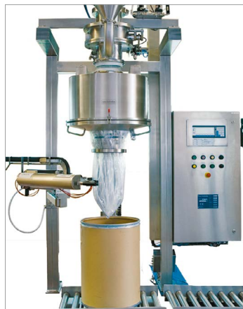
Endless-foil filling equipment with Vibro-Dos®, pneumatic clipper, balance and conveyor
