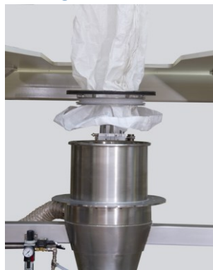
Pull the big-bag discharge spout through the sealing ring.
