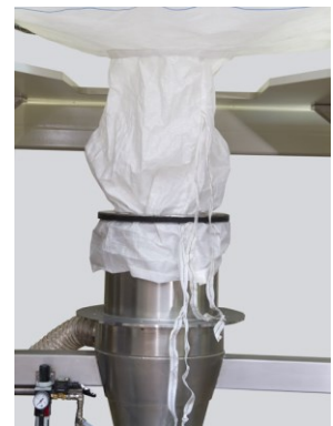
The sealing ring lowers, the inflatable seal tightens the system.
