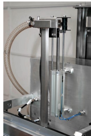
Welding machine with lowerable lance for headspace evacuation.
