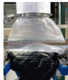
Weld the Containment-Foil and cut it with a separating welding seam
