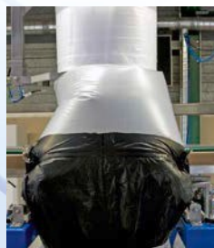
Open the welded seam with N2 pressure from inside or manually from outside (peel)
