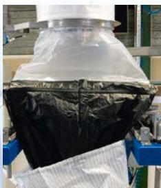
Insert the Containment-Foil into the Big-Bag In-Liner and weld
